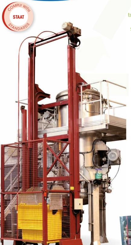
Our patented process is designed to shred and sterilize infectious waste by saturated steam. Shredding and sterilization are achieved in one fully enclosed and automated, stainless steel, system with no intermediate waste handling.
