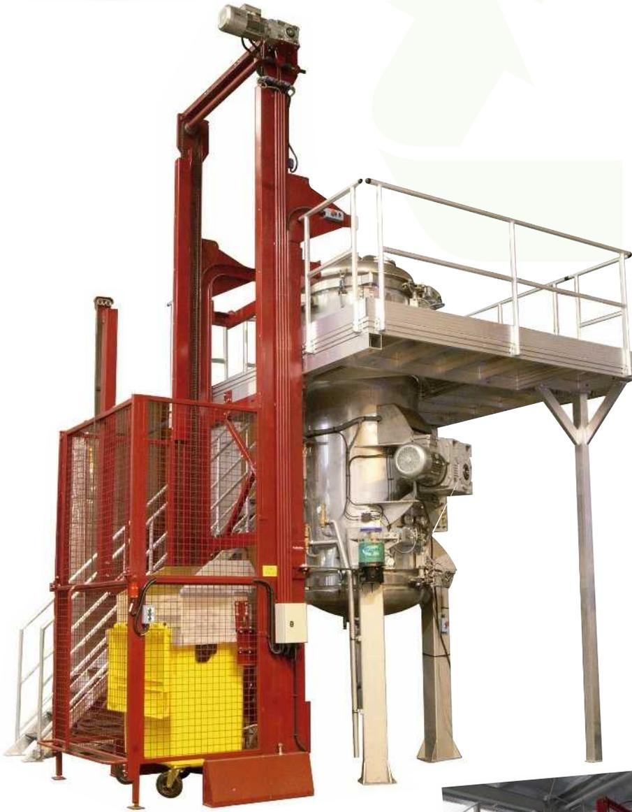
The contaminated waste is loaded into the upper chamber where a heavy-duty shredder reduces the waste into small pieces. Using gravity, the processed material drops into the lower treatment chamber.
