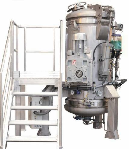
Our patented process is designed to **shred** and **sterilize** infectious waste by saturated steam. Shredding and sterilization are achieved in one fully **enclosed** and **automated**, stainless steel, system with no **intermediate** waste handling.
